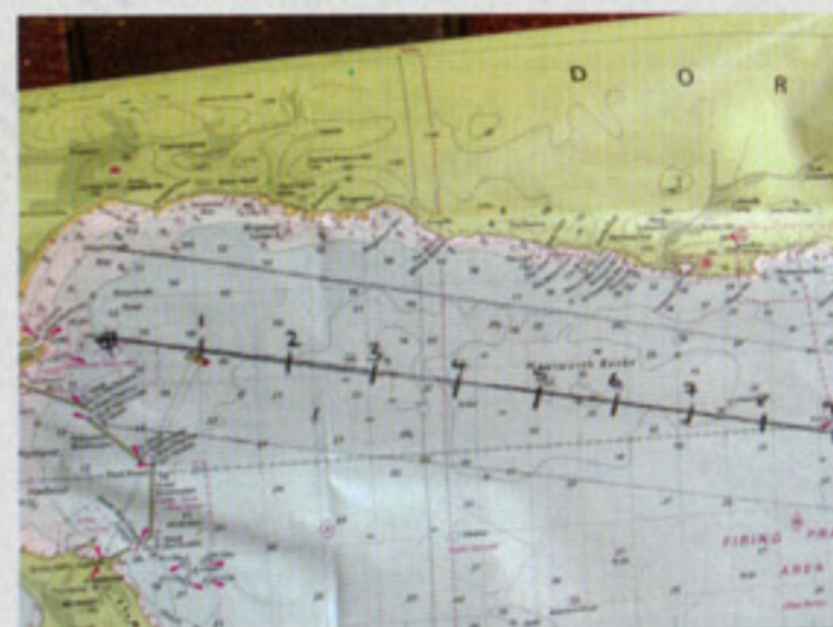
Draw the Waypoint Ladder between waypoints marking off 1m or 0.5m intervals, To each side mark lines at 1m, 2m etc - Distance to Go and XTE give a position.
