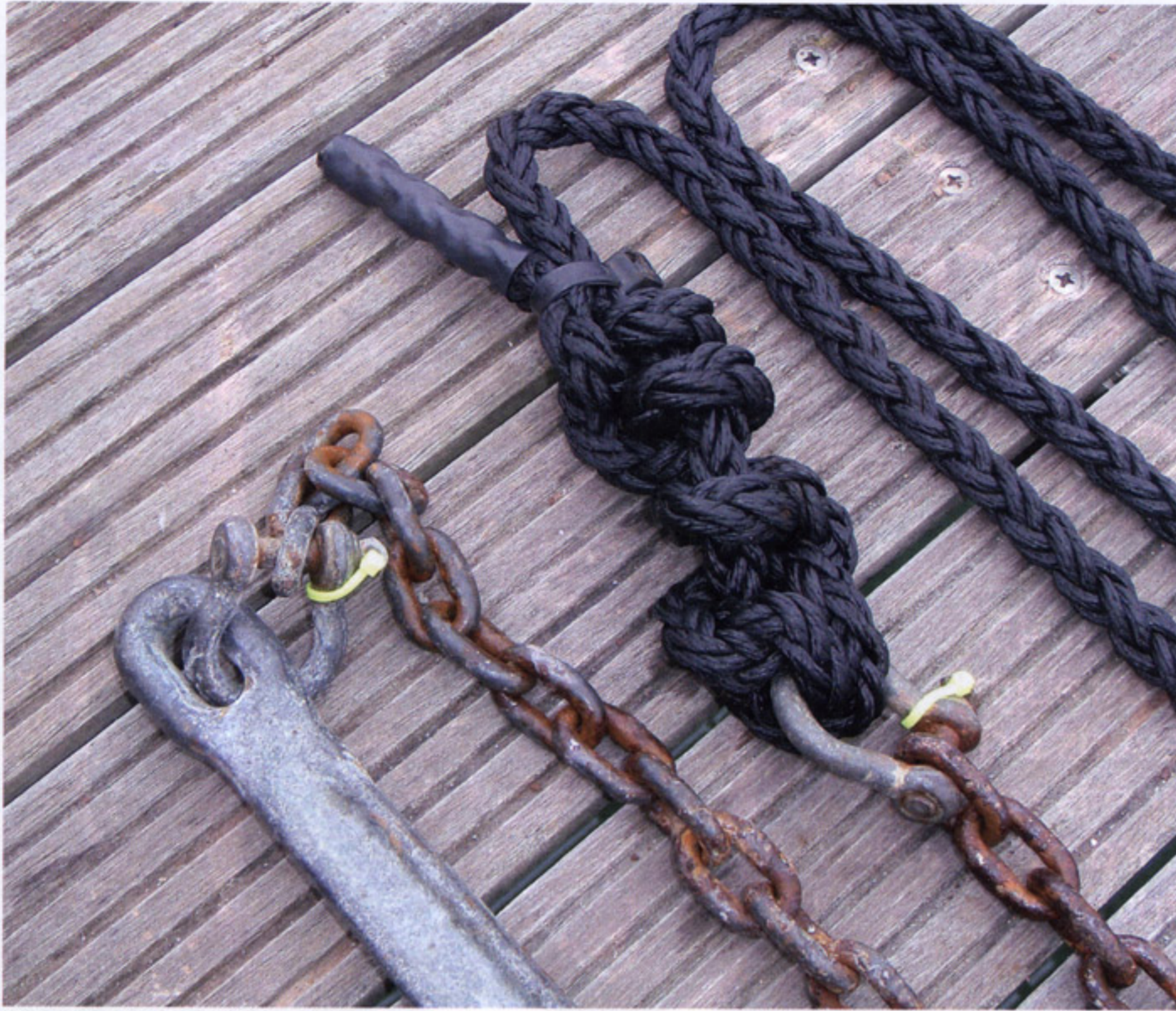
Methods of splicing and shackle attachment
