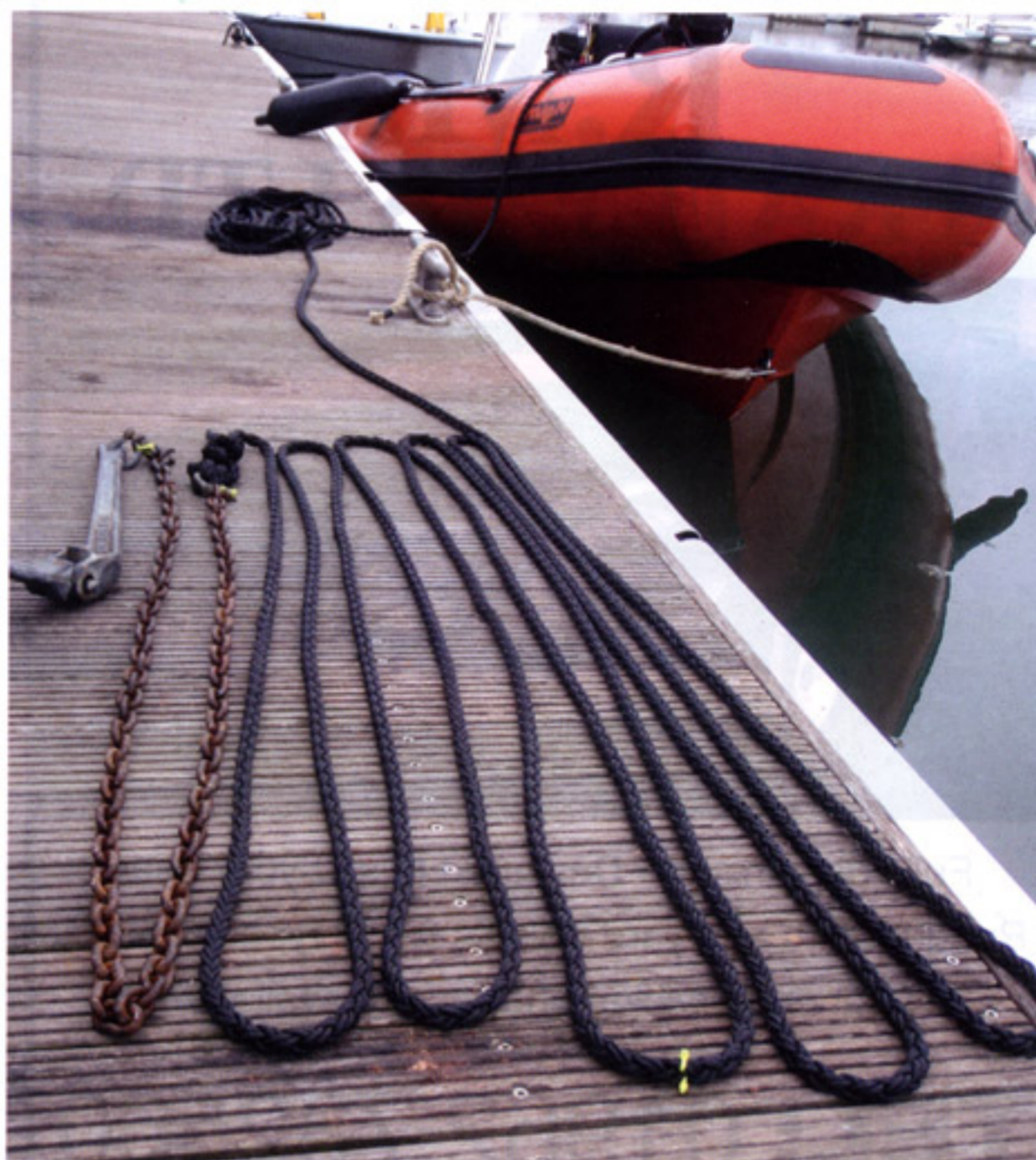
Note length of chain to length of rope, this is critical.
