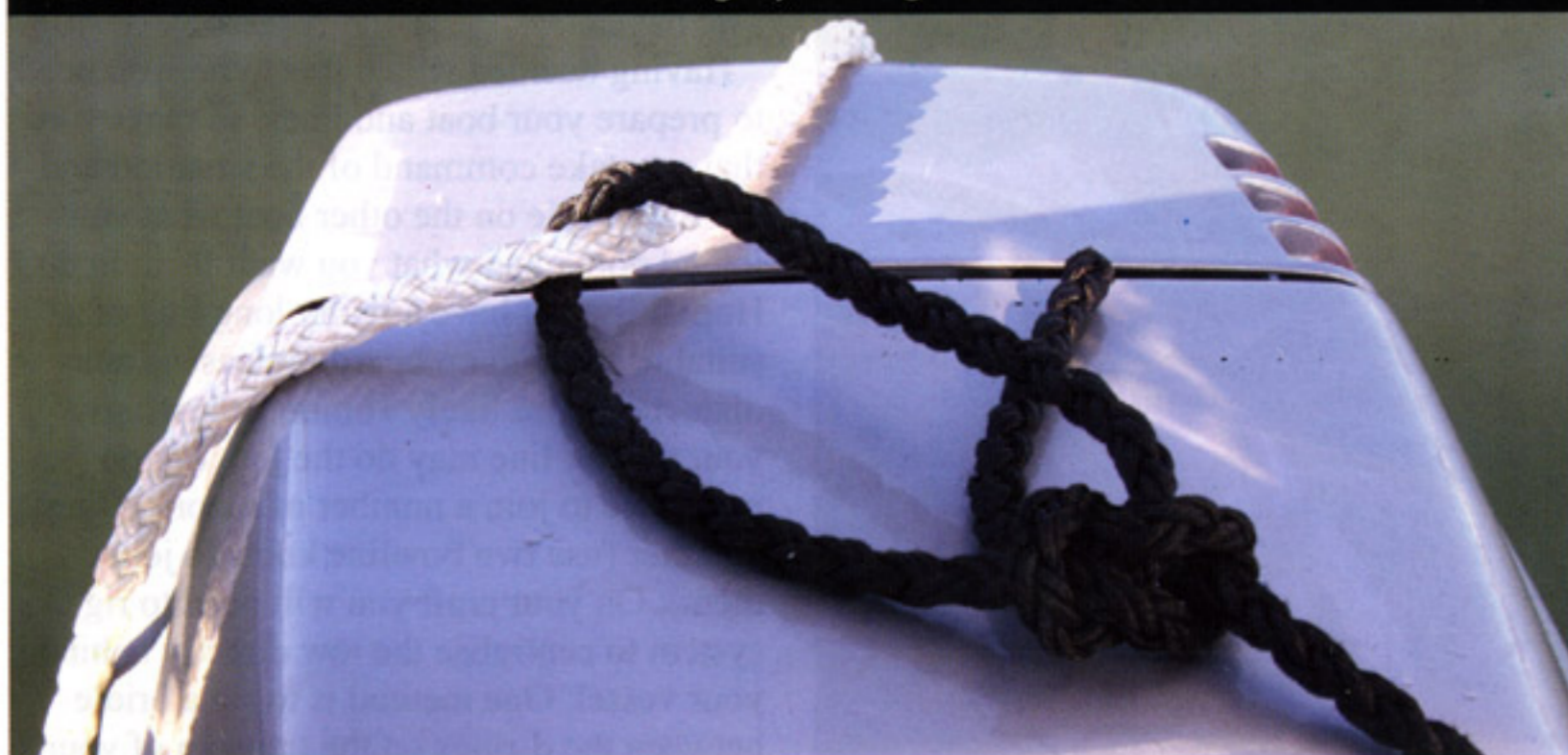
Long tow setup: The white line leads to the tricken vessel. The length of the tow line can be varied from within the 'tug' by easing out the white line.
